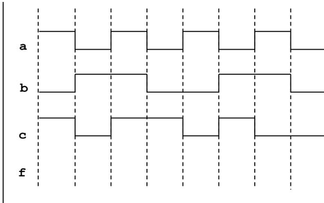
b) The following is the timing diagram of a logic circuit with 3 inputs. Sketch the logic circuit that generates this waveform. Then, complete the VHDL code. (10 pts)
